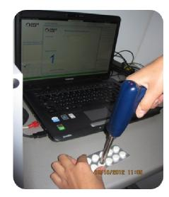
The pilot project for screening the quality of medicines with the Near Infra Red Spectrometry based on the mobile express laboratories; screening the quality of drugs using non-destructive method. These mobile labs are operating in all Federal Districts of the Russian Federation.
